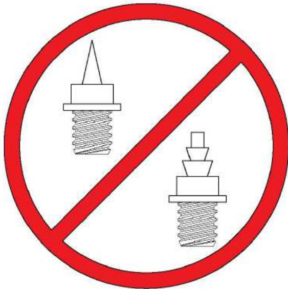
DAMAGING STEEL SPIKES
